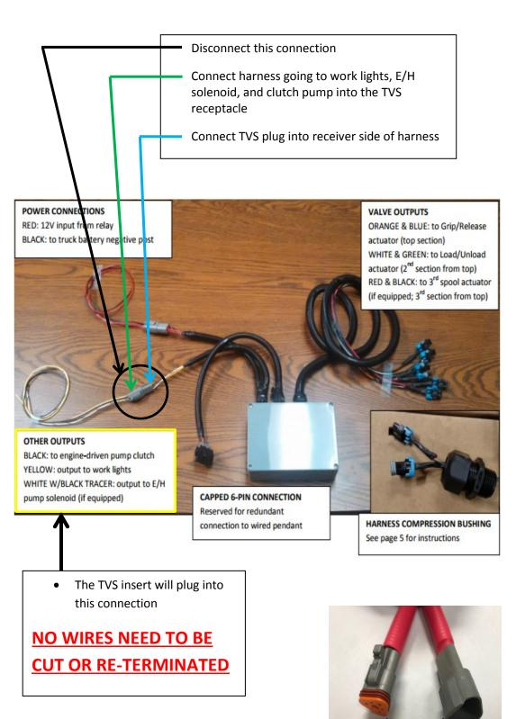
The TVS insert has a plug and receptacle allowing for plug and play
